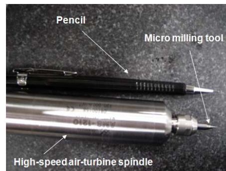
Fig. 3. The applied micro-cutting tool with a high-speed spindle.
